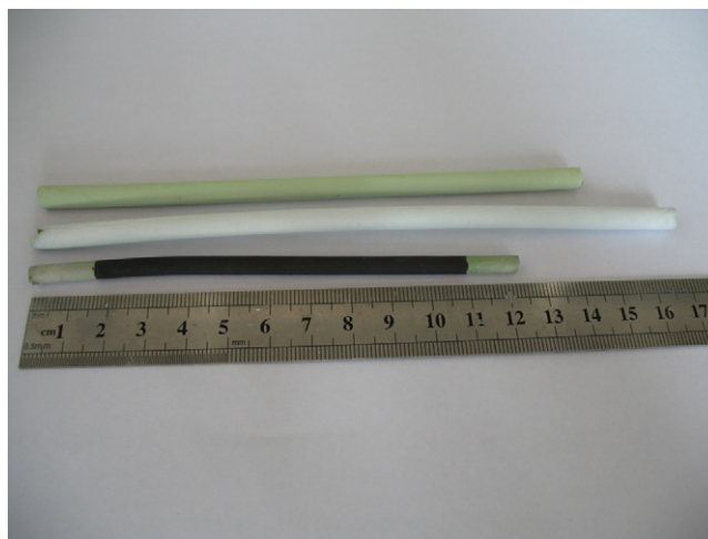
Fig. 2. Photograph of contrast among the anode substrate, thin electrolyte-coated anode substrate and the whole tubular cell.
